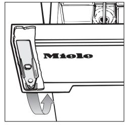
To clean the lint trap, remove the tool from behind the detergent dispenser drawer.
